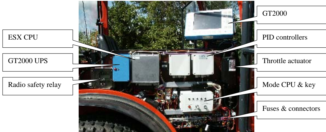
Figure 2. Hako tractor showing some of the retrofitted electronic components
