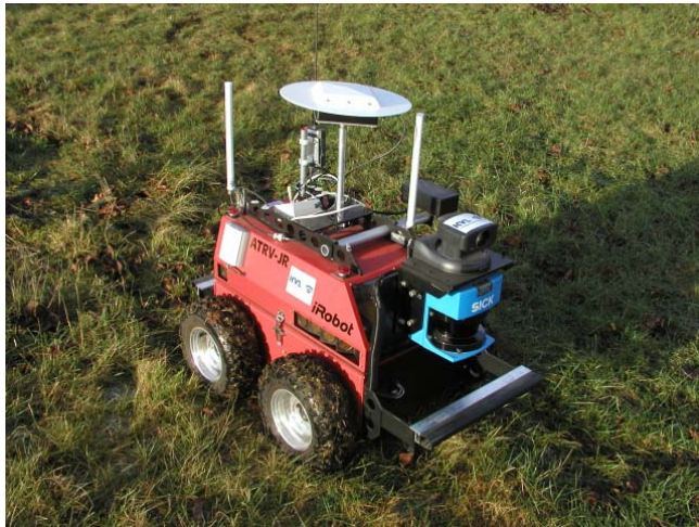
Figure 2. ATRV-jr from iRobot used in the tests
