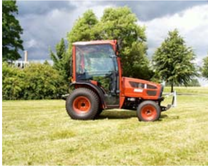
FIGURE 1. The Hakotrak 3000. This tractor is currently being adapted to accept the Agronav automatic steering system from GEO-TEC as part of a collaborative Danish research programme called Autonomous Platform and Information system (API).
