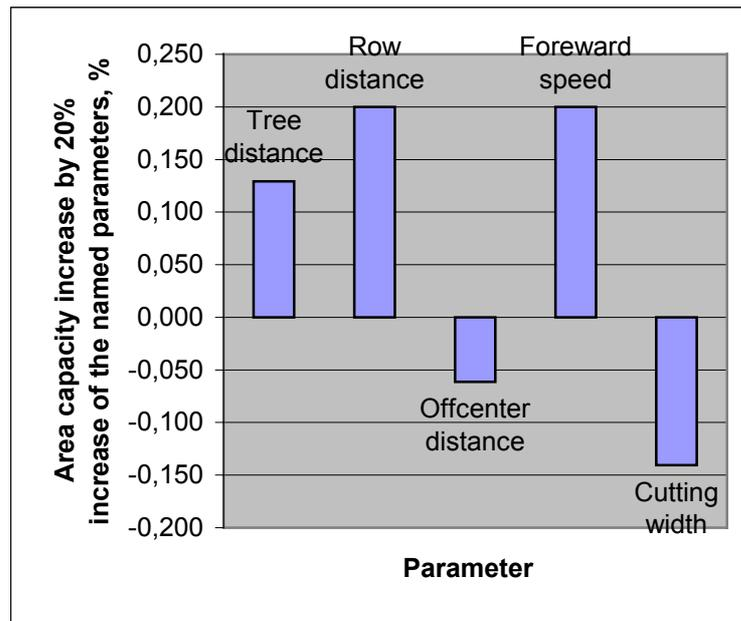
Figure 9.1. Sensitivity of the area capacity of weeding using an ACW in Loop operation pattern.
