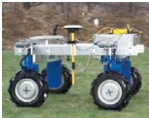
FIGURE 2. Small portal tractor from the Danish Technical University
