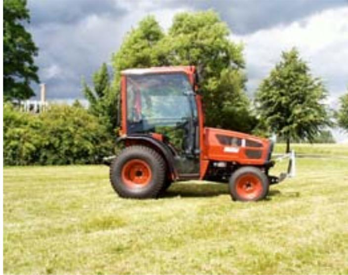
FIGURE 1. The Hakotrak 3000. This tractor is currently being adapted to accept the Agronav automatic steering system from GEO-TEC as part of a collaborative Danish research programme called Autonomous Platform and Information system (API).
