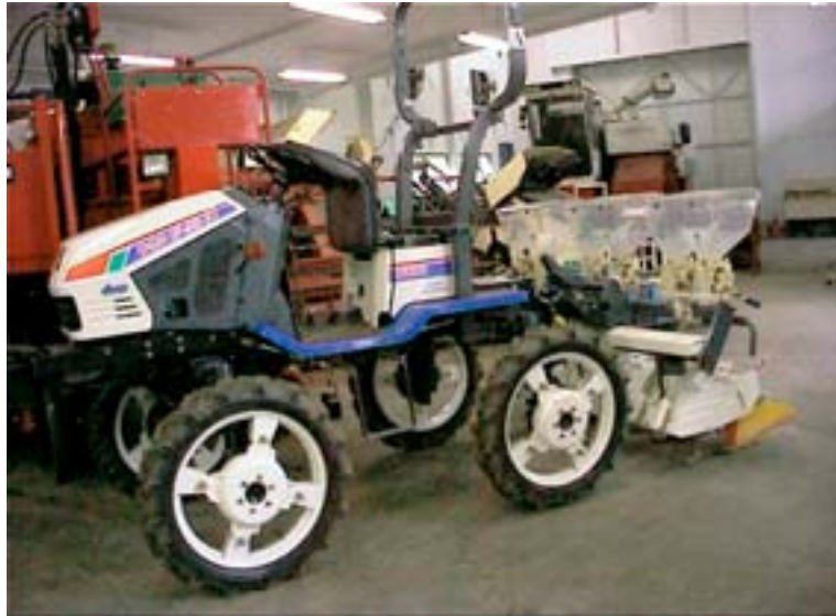
FIGURE 3. A Japanese, larger type, portal tractor.
