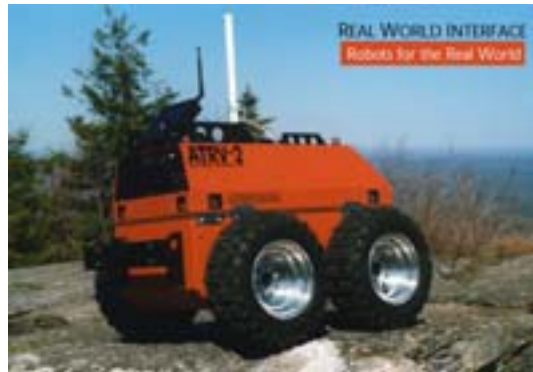
Figure 7.1: Example of skid steered commercial available autonomous vehicle platform for experiments. The unit is electric powered from batteries and fitted with basic sensors, computers and communication equipment, which are open for addition of supplementary units.
