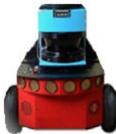
Figure 4. A small research vehicle with an ultrasonic and laser range finding systems
