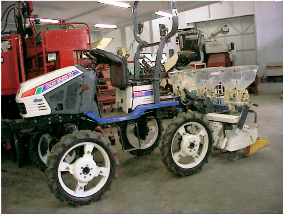
FIGURE 3. A Japanese, larger type, portal tractor.
