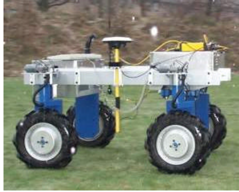
FIGURE 2. Small portal tractor from the Danish Technical University
